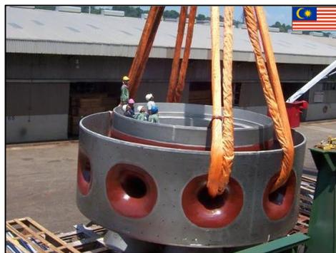
Unloading the "ATP Centre Support" section of the outer shell – a high alloy fabrication manufactured in **Malaysia**. Shipping weight was 164 tonnes.
