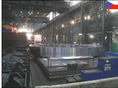
Casting and rough machining of the ATP support tyres was done in the **Czech Republic**. The tyres were shipped to China in 180° segments and welded together on site. Each tyre weighs 120 tonnes (note workers in behind the tyre).
