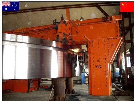
Field machining of the 11 m (36') diameter support tyres on-site by Self-Levelling Machines (SLM) of **Australia**.
